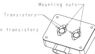
Step I: Tighten mounting nuts on transistors on bottom of FSD/PMD.
